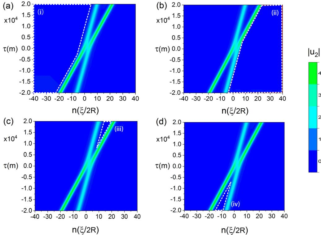
FIG. 6. The double soliton solution Eq. (18) shown by the areas marked with the dashed lines [(i), (ii), (iii), and (iv)] corresponding to four conditions: (a)  $e^{\theta_1}, e^{\theta_2} \gg 1$ ; (b)  $e^{\theta_1}, e^{\theta_2} \ll 1$ ; (c)  $e^{\theta_1} \gg 1, e^{\theta_2} \ll 1$ ; (d)  $e^{\theta_1} \ll 1, e^{\theta_2} \gg 1$ . The parameters and the meaning of the highlighted areas are the same as described in the caption of Fig. 3.
