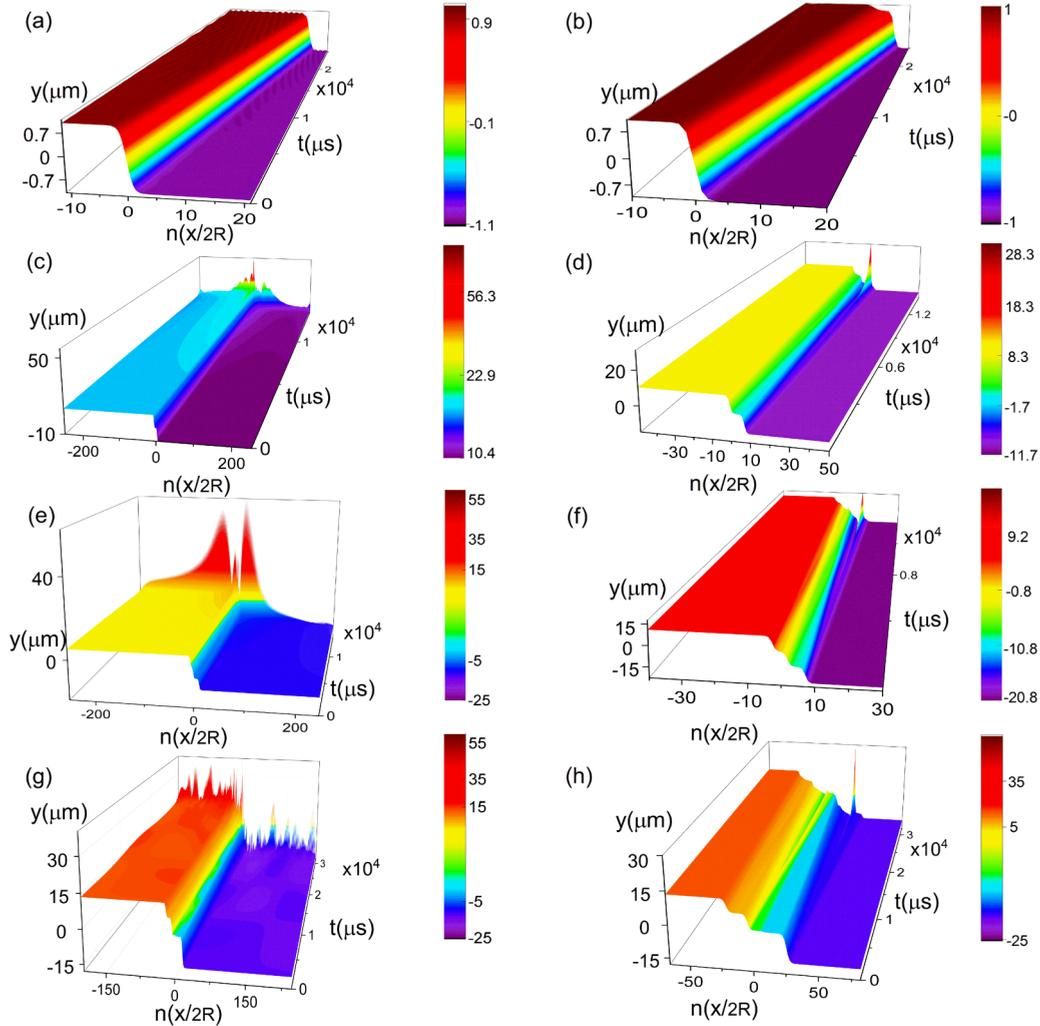
FIG. 10. Numerical simulation of the solitary waves inspired by a perturbed excitation at  $t = 0$  with the parameters listed in Table II: (a), (c), (e), and (g) show evolution of the single, double, triple, quadruple dark solitary waves from Eq. (9) simulated by SSFT method; (b), (d), (f), and (h) show evolution of the single, double, triple, quadruple dark solitary waves from Eq. (6) simulated by Runge-Kutta method.
