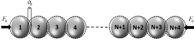
FIG. 1. Schematic diagram of the granular chain of elastic spheres precompressed by a static load.
