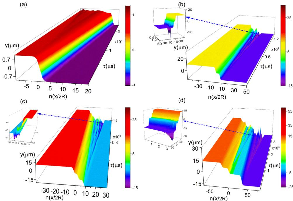
FIG. 11. Evolution of the single (a), double (b), triple (c), and quadruple (d) dark solitary waves simulated from Eq. (4) inspired by a perturbed excitation at  $t = 0$  with the same parameters as in Fig. 10 by using Runge-Kutta method.
