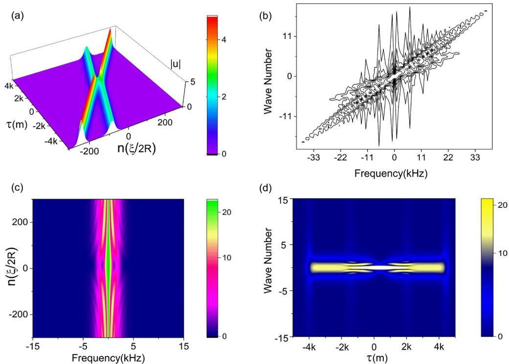
FIG. 8. Evolution of the double solitary wave solution Eq. (18) in the space-time domain (a) and wave-number-frequency domain (b). Panel (b) can also be viewed as the dispersion curve corresponding to panel (a); panels (c) and (d) show the energy transfer during the dynamic collision process in the time-wave-number domain and space-frequency domain, respectively.
