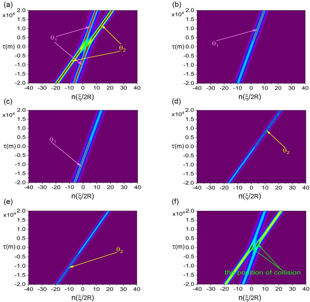
FIG. 3. Intensity profiles of the double-soliton solution Eq. (18) (a) and approximate solutions Eqs. (21)–(24) (b–e, respectively) with the highlighted areas corresponding to limiting cases (i)–(iv) where  $\beta = 4887 \mu\text{m}^2$ ,  $R = 2 \text{ mm}$ ,  $k_1 = 1 \text{ m}^{-1}$ , and  $k_2 = 1.4 \text{ m}^{-1}$ .
