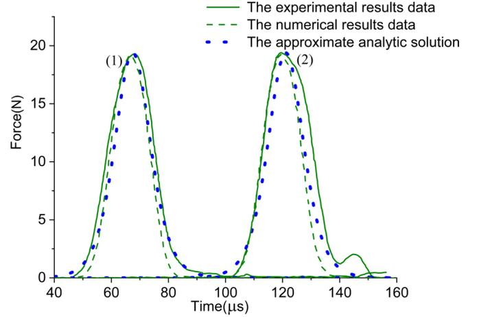
FIG. 14. Comparison between the present approximate analytical solutions with the experimental and numerical results in Fig. 3 of Ref. [80]: forces between the 7th and 13th particles in the chain of cylindrical particles with  $\alpha = 90^\circ$ .
